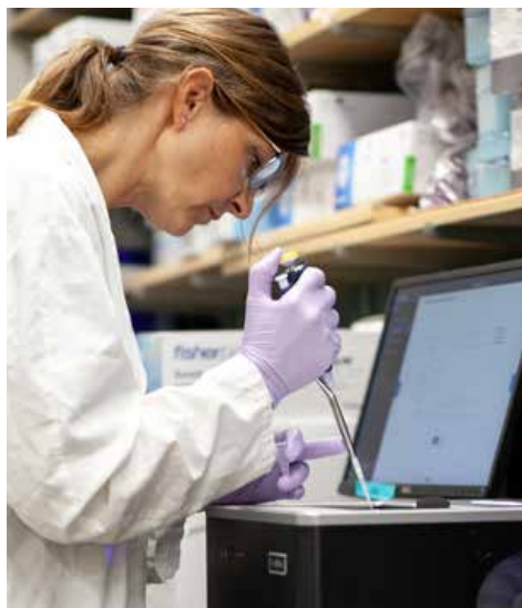
Loading a sequencing library on to a GridION flow cell.
